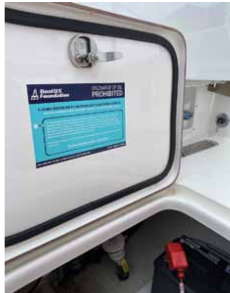
The BoatUS Foundation oil discharge placard decal on machinery spaces, such as a bilge access door, helps ensure proper handling of oil waste.
